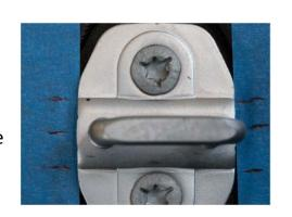
Open your tailgate and place the assembled locker into the jeep sliding the notch in the wall between the latch plate and the tub frame.
